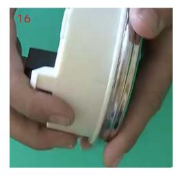
Reinstall the gauges in the bezel or inner fairing. Re-install the bezel (if applicable) and replace all clamps and screws that were previously removed.
