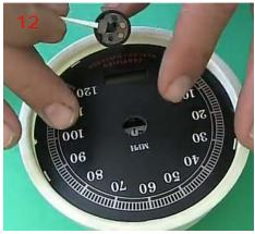
With the needle removed, use a suitable tool (flat head screwdriver or small pick) to get under the outside edge of the factory gauge face (13). If you plan to save these for possible reinstallation, take caution as they are very thin. Pry up on the gauge face until you separate it from the internal base of the gauge. It is held down by adhesive so this make take some time to work around the whole gauge face and remove it. (14)
