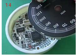
With the factory faceplate removed you can now install the new Speed Gauge Customs faceplate. Align the small tabs in the faceplate with the indentions in the internal gauge base (15).
