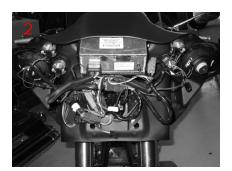
**Street Glide models** – With the outer fairing removed begin by unplugging the two large gauges (speedometer and tachometer (3). Next, remove the mounting brackets that secure the gauges to the inner fairing (4).
