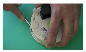
Once you have gone all the way around the gauge, do the same procedure again but focus on making the top edge of the chrome ring the same diameter as the lip on the white plastic housing (9).
