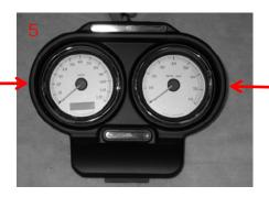
Remove the gauge housing cover by lifting and pulling forward to remove the tab from under the ignition switch (6).
