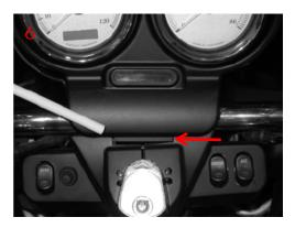
Unplug the gauges and indicator lights from the wiring harness and completely remove the gauges and bezel from the bike. Remove the clamps holding the gauges to the bezel and set them aside.
