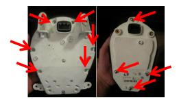
5. Remove the 2 screws that hold the faceplate to the clear plastic base inside the speedometer
