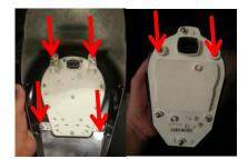
4. Remove the screws\* that secure the white backing plate to the black front cover and glass.
