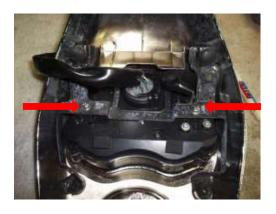
5) Remover two (2) long thin silver screws – reset switch wires
