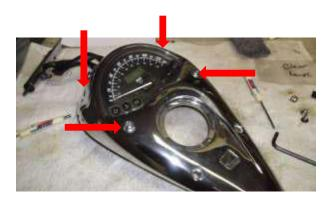
4) Remove two (2) short silver screws – separate speedometer assembly from bracket.
