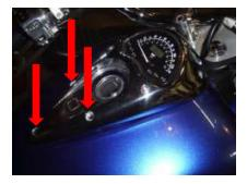
Remove gas cap, lift rear of assembly up over gas neck and then entire assembly forward.
