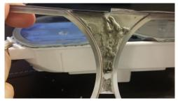
4. Now that you have access to the glass covers, begin by removing the 3 star screws indicated by red arrows below using a T9 star bit.
