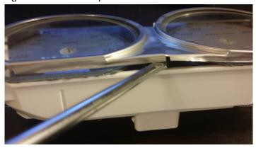
3. Push up towards the top as far as you can, being careful not to hit the glass. Once you have loosened the double sided tape that holds this down you can pull up on the edges all the way around the gauges and the entire piece will lift off. Be patient, this can take a little bit of time.
